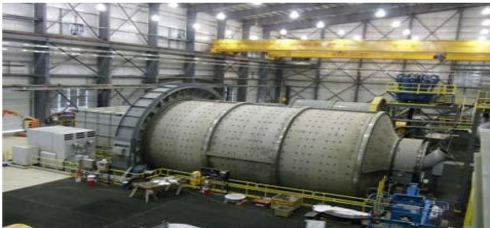
Figure 1. The ball mill machine
