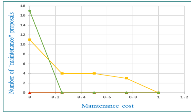
Figure 3. The effect of changes in maintenance cost on the number of maintenance proposals as the optimal policy in each period of planning horizon (Red: First period, Orange: Second period, green: Third period)
