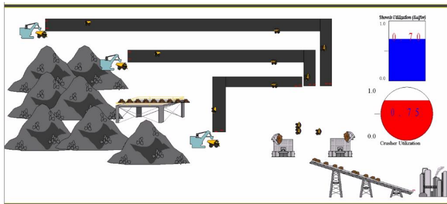
Figure 2. Animation of the haulage system at Sarcheshmeh copper mine in Arena software
