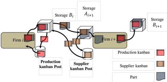
Figure 1. Kanbans operations between two firms.
